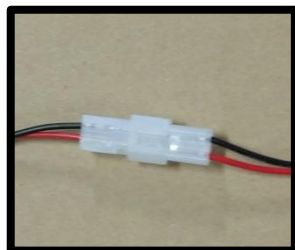
3) Both Photocell extension cables connected
